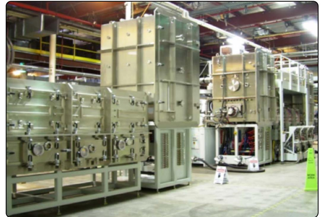
**Figure 4** – Large-scale CIGS Deposition Tool Capable of Processing 1 m Wide Web to be Installed at USPVMC Manufacturing Development Facility
